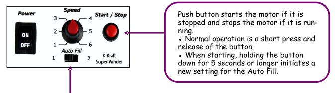
Auto Fill stops the motor after a preset number of revolutions. There are 2 choices, allowing for the use of 2 different size bobbins. The settings can be easily changed and will be retained until there is a new setting. Auto fill is always active, initially we set it very high so you will want to <u>set it for your bobbin.</u>
